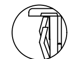
DETAIL VIEW VH1 HOLE PLUG (No wing serrations for ease of removal)
